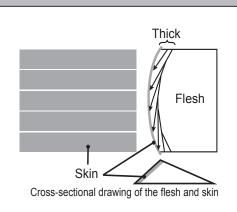
Adjusting the unit to take a thicker peel increases the number of overlapping passes of the blade, thereby increasing the amount of peel removed. The peeler blade passes over the fruit more slowly, leaving less peel.
