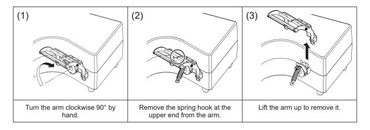
• To attach the arm, place the two holes at the base of the arm over the two pins on the arm holder, then attach the hooked end(s) of the spring(s) to the groove(s) on the arm shaft.
