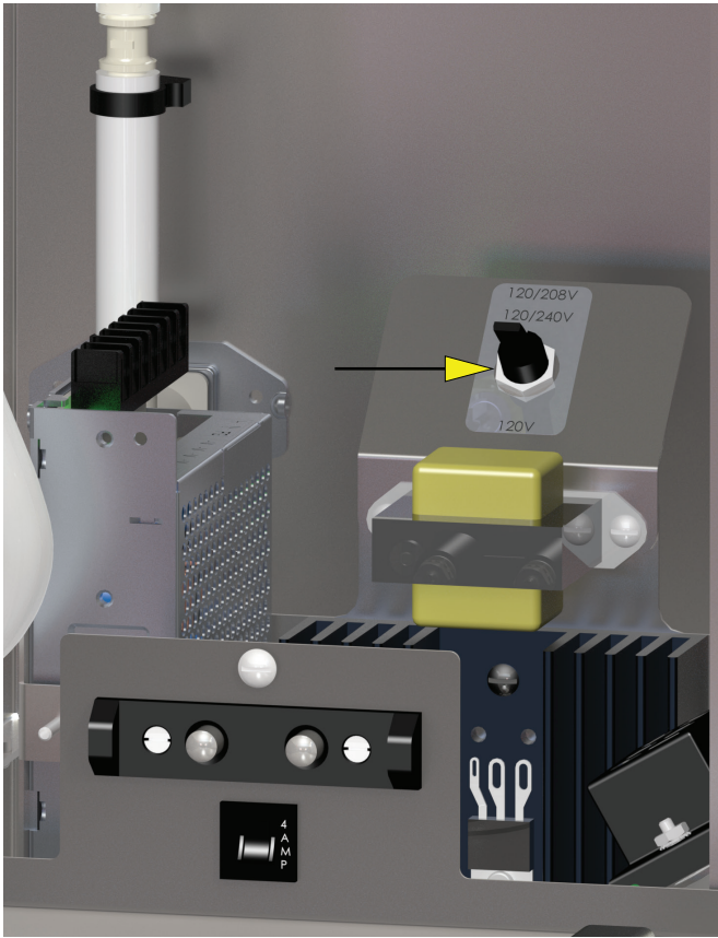
FIG. 21-1 VOLTAGE SELECTOR SWITCH
